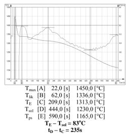
Fig. 9. ATD analysis curve plotted for the IN-713 C alloy (ingot with shrinkage cavities)
