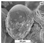
Fig. 5. Dendrites coated with oxides near the shrinkage cavity in a master heat ingot made from the IN-713C alloy
