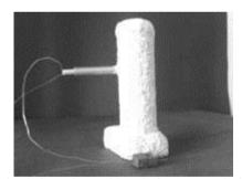
Fig. 4. Ceramic mould ready for ATD analysis
