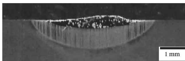
Fig. 17. Surface layer of the 32CrMoV12-28 steel after alloying with WC, the laser power of 2.0 kW
