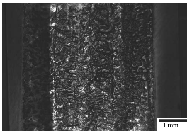
Fig. 26. Wear trace of the surface layer after an abrasion test acc. to ASTM G65 for the X40CrMoV5-1 steel alloyed with the WC tungsten carbide powder, laser power of 1.2 kW
