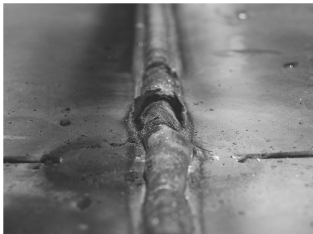
Fig. 4. Weld distortion by over-pressure jet cooling
