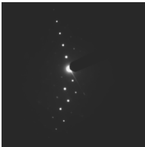
Fig. 12. Diffraction pattern of the particle in Fig. 10
