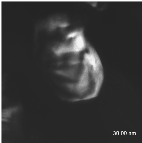
Fig. 11. Mg 2 Si phase microstructure, bright field, TEM
