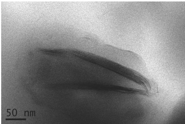
Fig. 48. Intercalation of MMT galleries approved by transmission electron microscopy
