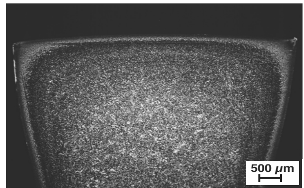
Fig. 23. Cross section of the neat PP specimen performed by CIM in 280°C
