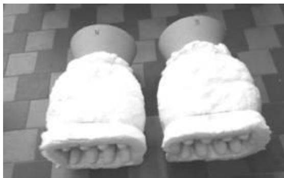
Fig. 3. Moulds with insulation ready for tests
