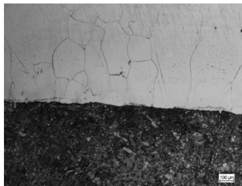
Fig. 6. Microstructure of joint area between austenitic alloy steel and ferritic-pearlitic unalloyed cast steel C = 0,55% at T_{zal} = 1600^{\circ}\text{C} – etching Mi19Fe
