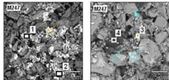
Fig. 6. Microstructure and chemical composition of precipitates present in zone I of „blue” mould poured with MAR-247 alloy
