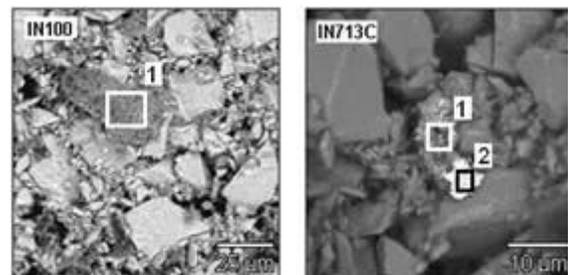
Fig. 5. Microstructure and chemical composition (EDS) of precipitates present in zone 1 of „blue” mould poured with Inconel alloys
