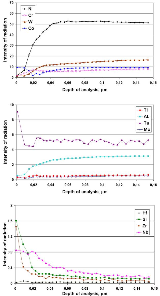
Fig. 8. Concentration of constituents in surface layer of MAR-247 alloy casting („blue” mould)
