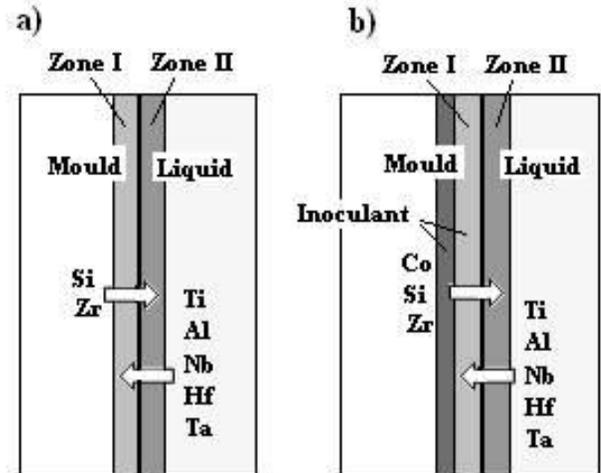
Fig. 1. Schematic representation of chemical interactions at the interface of: a) mould material-molten alloy, b) modifying coating-molten alloy
