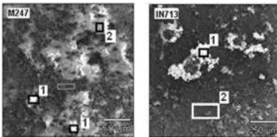
Fig. 7. Microstructure and chemical composition of precipitates present on the raw surface of castings made from MAR-247 and IN-713C alloys („blue” mould)
