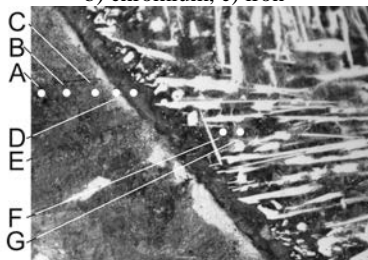
Fig. 11. Microhardness measurements location (magnification 400x); A-C) cast steel, D) decarburization zone, E) transition zone, F-G) alloy layer
