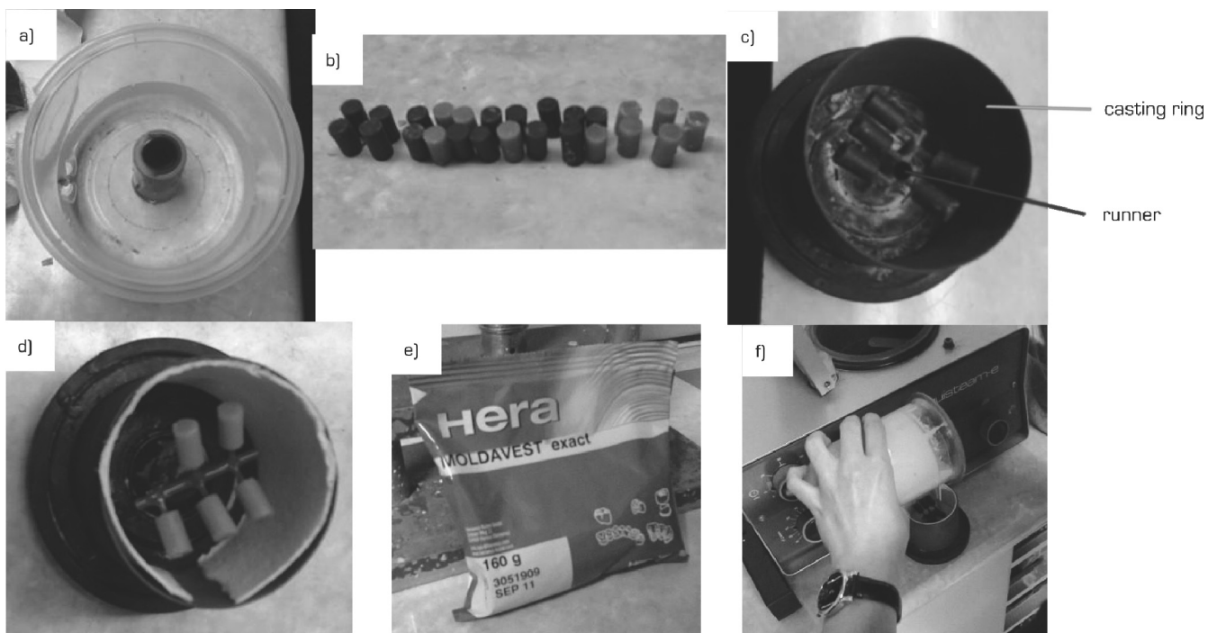
Fig. 2. Stages of preparing the mould to cast tests specimens: a) preparing the wax model by cast liquid wax into silicon mould placed in cold water, b) wax specimens after remove from silicon and cut, c) wax models with runners in casting ring, d) paper band install to better expansion of investment material, e) the investment materials to prepare the mould, f) fill the casting ring by investment material after vacuum mixing
