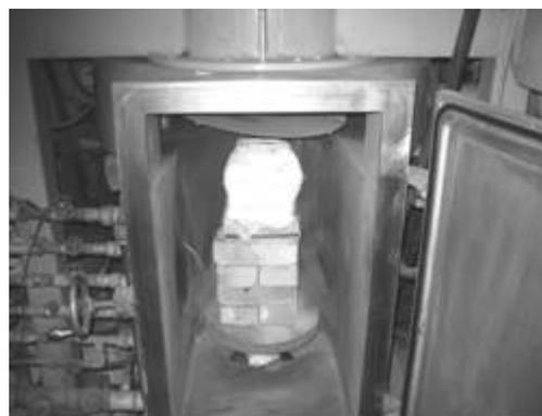
Fig. 2. Preheated mould in the chamber of induction furnace made by Leybold
