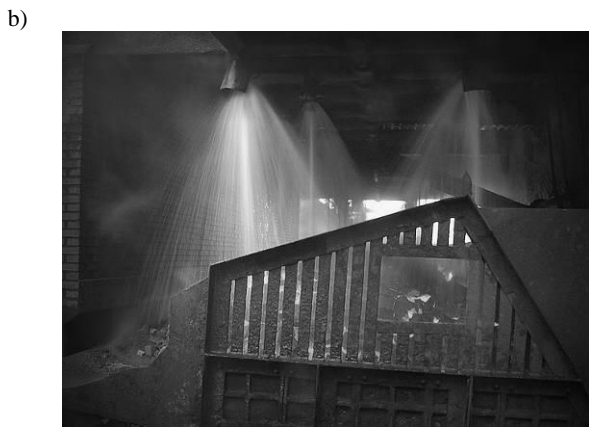
Fig. 1. View of quenching car with lining in form of cast iron plates in time of following stages of work: a) dropping of heated coke and b) its quenching [7]
