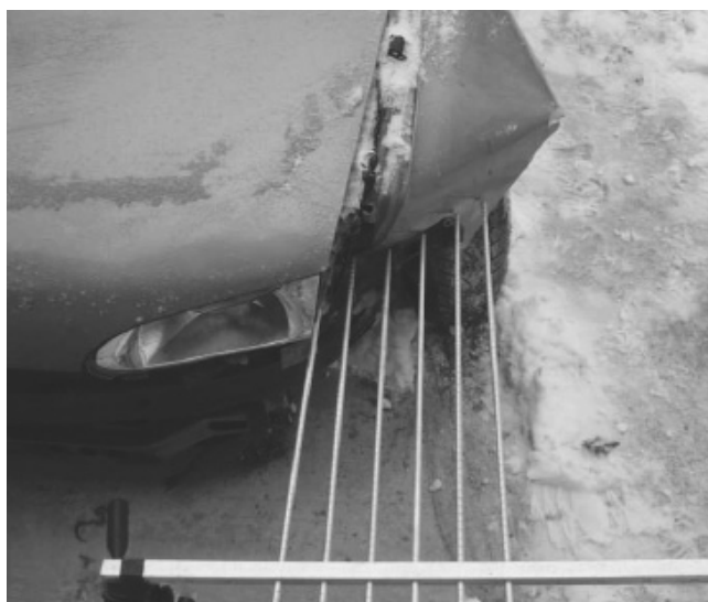
Fig. 14. Deformation of Hyundai Accent 1995, impact speed of 16 km/h, maximum deformation of 0.31 m
