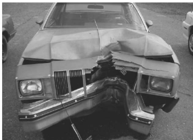
Fig. 6. Deformation of Oldsmobile Cutlass 1978, impact speed of 45 km/h, maximum deformation of 0.64 m [18]
