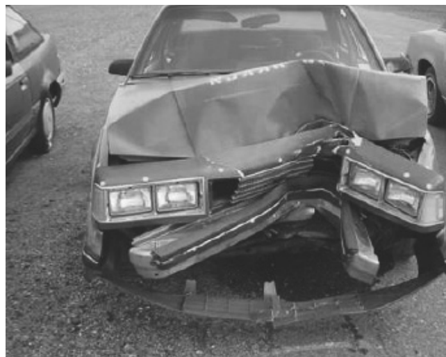
Fig. 8. Deformation of Chevrolet Celebrity 1986, impact speed of 49 km/h, maximum deformation of 0.55 m [18]
