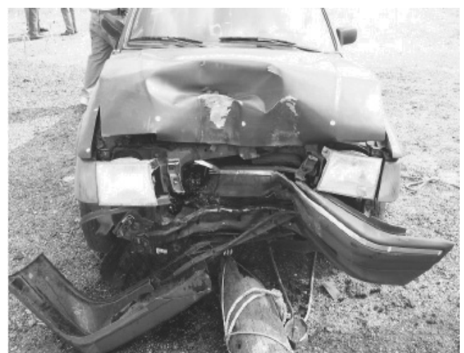
Fig. 10. Deformation of Ford Escord 1989, impact speed of 47 km/h, maximum deformation of 0.43 m [18]
