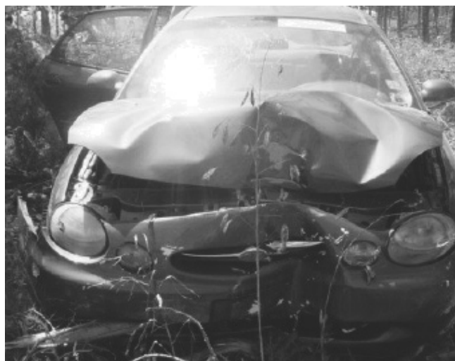
Fig. 12. Deformation of Ford Taurus 1999, impact speed of 78 km/h, maximum deformation of 0.39 m [18]
