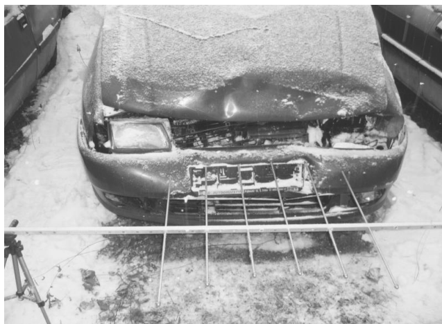
Fig. 16. Deformation of Seat Cordoba 1997, impact speed of 18 km/h, maximum deformation of 0.26 m
