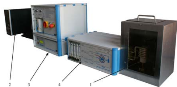
Fig. 1. UMSA apparatus - (1) sample chamber, (2) supervisory computer, (3) temperature control, (4) gas flow control
