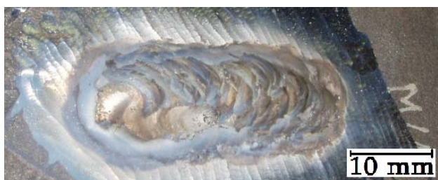
Fig. 8. Fragments of repair of side wall of huge-dimensions cast of sump gear of aviation engine - face of weld, b) macrostructure of the padded area.
