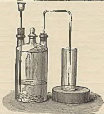
Apparatus for the preparation and collection of carbonic acid gas.
