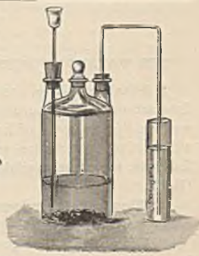
Showing how a solution of carbonic acid gas may be prepared.
