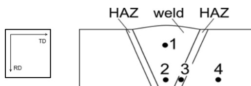
Fig. 2. The areas of microstructural studies in the welded joint and the arrangement of particular zones (1 - the weld, middle; 2 - the weld, root; 3 - the heat affected zone HAZ; 4 - the parent metal PM)
