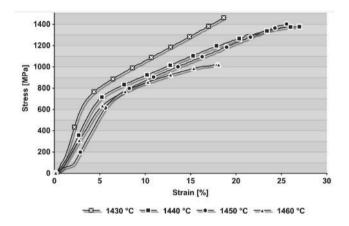
Fig. 11. Compression strength curves after different casting of the Remanium 2000+ alloy
