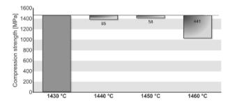
Fig. 15. Influence of casting temperature on compression strength of the Remanium 2000+ alloy
