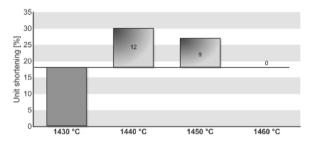
Fig. 17. Influence of casting temperature on shortening of the Remanium 2000+ alloy
