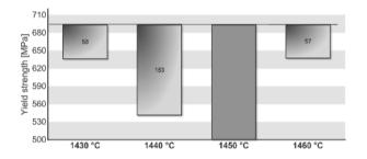
Fig. 14. Influence of casting temperature on yield strength of the Wirobond LFC alloy
