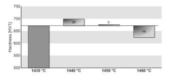
Fig. 9. Influence of casting temperature on hardness of the Remanium 2000+alloy
