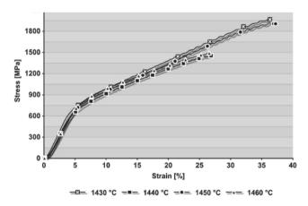
Fig. 12. Compression strength curves after different casting of the Wirobond LFC alloy
