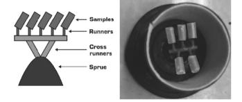
Fig. 1. The prepared model and mould to casting
