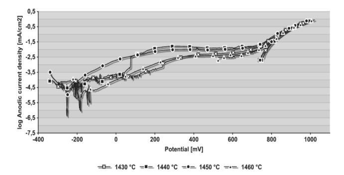
Fig. 7. Potentiodynamic curves of pitting corrosion Remanium 2000+ alloy after four different casting temperature
