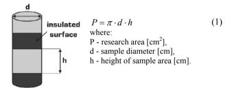
Fig. 3. Sample prepared to electrochemical test
