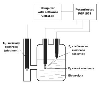
Fig. 4. Scheme of the corrosion resistance set to evaluate pitting resistance
