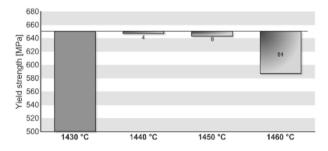
Fig. 13. Influence of casting temperature on yield strength of the Remanium 2000+ alloy
