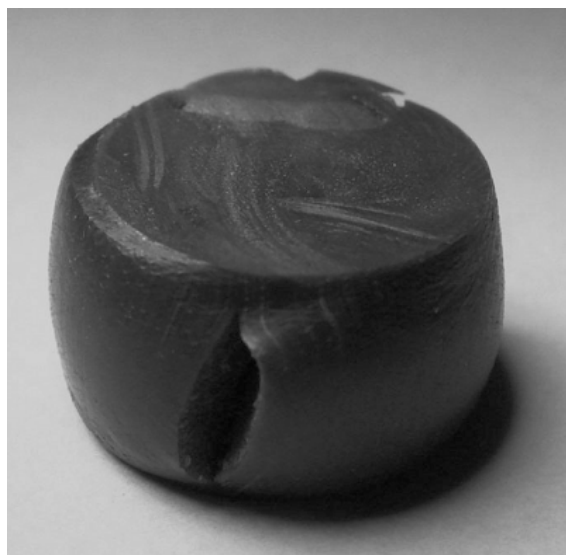
Fig. 12. Photograph of damaged test sample - Epidian 6 + Z1 (40% wt.) - Wood's alloy (60% wt.) composite
