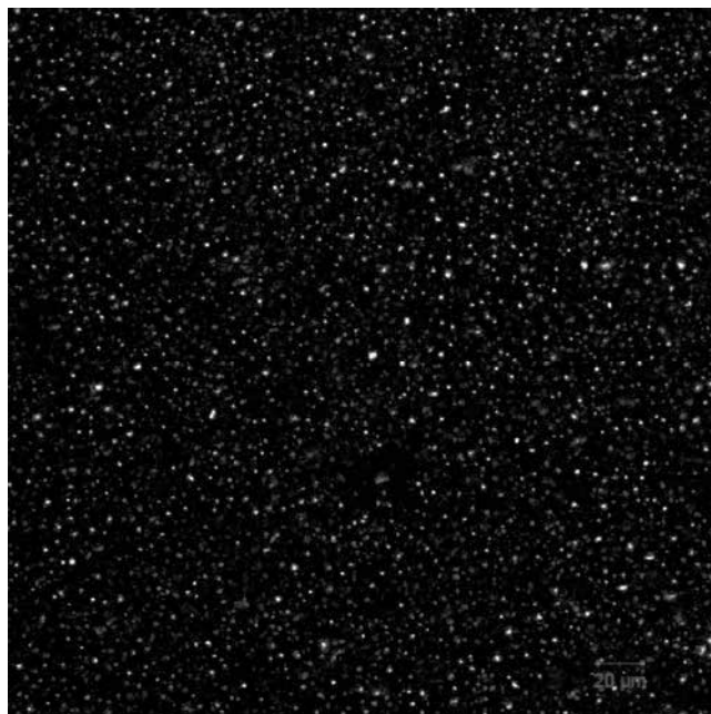
Fig. 5. Exemplary microscopic image of - Epidian 6 + Z1 (20% by weight) - Wood's alloy (80% by weight) composite
