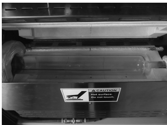
Fig. 6. Quartz process pipe situated in the oven
