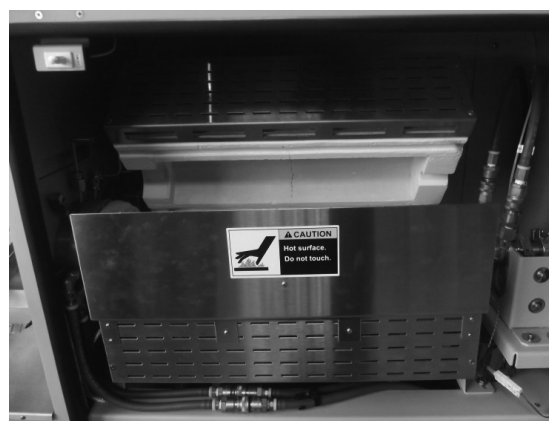
Fig. 5. Oven situated in the central unit allowing to reach process temperature of 1100°C
