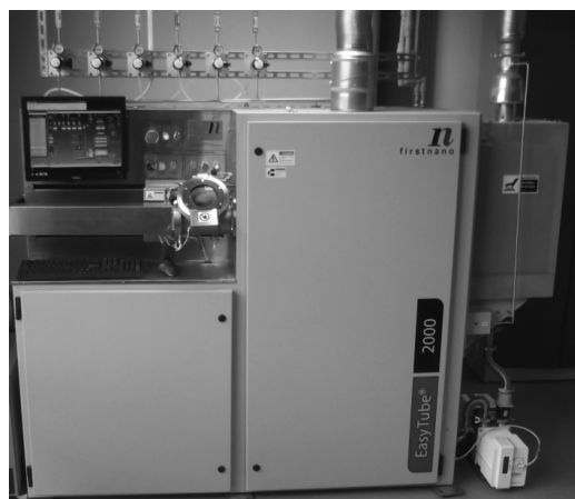
Fig. 3. EasyTube® device by FirstNano used for carbon nanotubes synthesis
