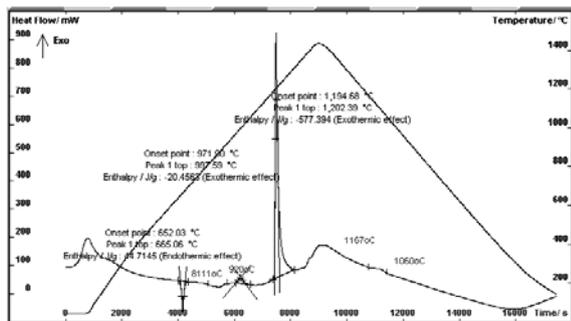
Fig. 6. DSC curve plotted for a mixture of  $\text{CoAl}_2\text{O}_4 + 10\%$  Al powder + colloidal silica
