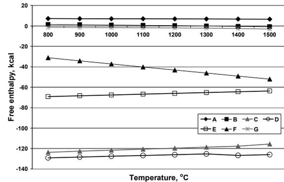
Fig.1. Free enthalpy in function of temperature for reactions included in groups 1 and 2
