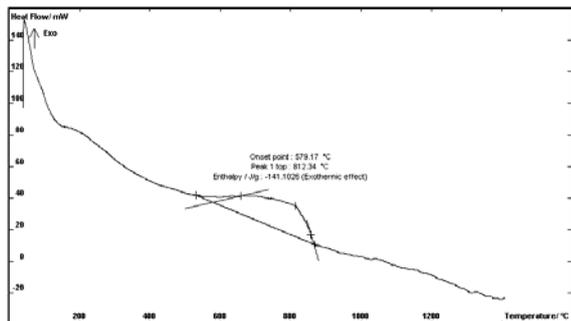
Fig. 4. DSC curve plotted for cobalt aluminate  $\text{CoAl}_2\text{O}_4$
