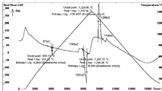
Fig. 8. DSC curve plotted for a system of  $\text{ZrSiO}_4$  coating +  $10\%$   $\text{CoAl}_2\text{O}_4$  on IN-713C alloy sample
