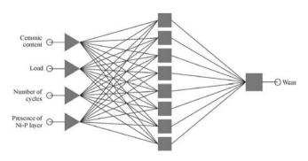
Fig 4. The scheme of neural network MLP 4-8-1 used modeling of tribological properties of composite materials
