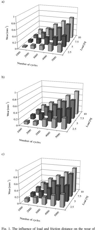
Fig. 1. The influence of load and friction distance on the wear of obtained composite materials with different ceramic content (uncoated reinforcement): a) 31%, b) 25% and c) 20%
