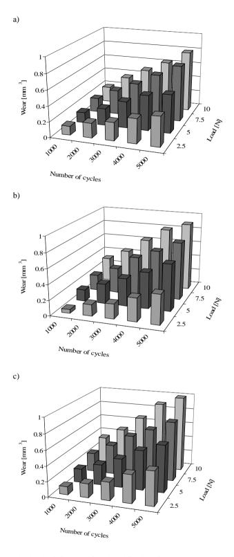
Fig. 2. The influence of load and friction distance on the wear of obtained composite materials with different ceramic content (reinforcement coated by Ni): a) 31%, b) 25% and c) 20%.
