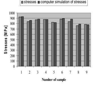
Fig. 12. Comparison of computer simulation with results of experimental investigations for stresses of TiN coatings
