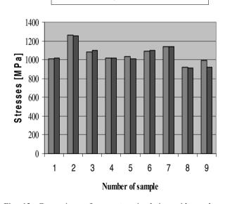
Fig. 13. Comparison of computer simulation with results of experimental investigations for stresses of TiC coatings
