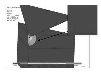
Fig. 4. Deformation and distribution of tensions in TiN coat (thickness of coat g=2.2  $\mu$ m, temperature of process 540°C)
