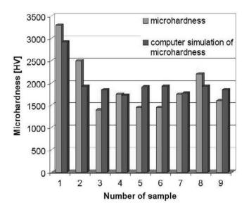
Fig. 10. Comparison of computer simulation with results of experimental investigations for microhardness of TiN coatings
