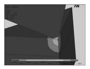
Fig. 5. Distribution of tensions in TiC coat (thickness of coat  $g=2.6 \mu m$ , temperature of process 540°C)
