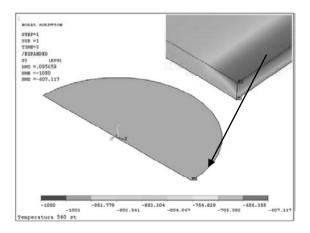
Fig. 6. Distribution of the simulated compression stresses in the TiN coating (coating thickness g=4.6 µm, process temperature 540°C, specimen distance from the magnetron disk 95 mm)
