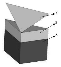
Fig. 1. Model of the sample: A - Substrate (ASP 30), B - Coating (TiN, TiC), C - Indenter Model Surface
