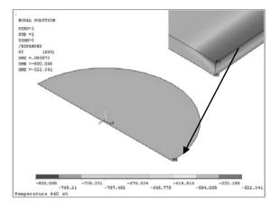
Fig. 7. Distribution of the simulated compression stresses in the TiN coating (coating thickness g=3.9  $\mu$ m, process temperature 460°C, specimen distance from the magnetron disk 125 mm)
