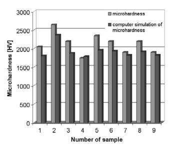
Fig. 11. Comparison of computer simulation with results of experimental investigations for microhardness of TiC coatings
