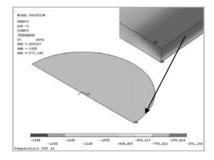
Fig. 9. Distribution of the simulated compression stresses in the TiC coating (coating thickness g=2.6 µm, process temperature 500°C, specimen distance from the magnetron disk 125 mm)
