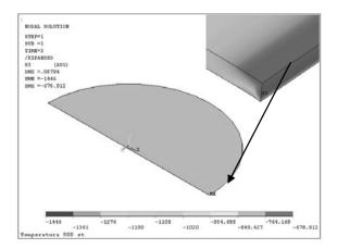
Fig. 8. Distribution of the simulated compression stresses in the TiC coating (coating thickness g=2.6 µm, process temperature 540°C, specimen distance from the magnetron disk 95 mm)
