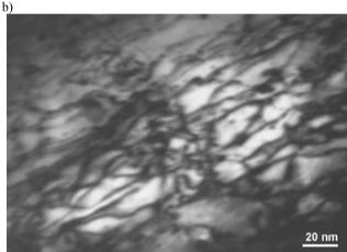
Fig. 8. Dislocation cells in CRS processed CuCr0,6 alloy strips: athin foil parallel to the strip surface, b- thin foil perpendicular to the strip surface
