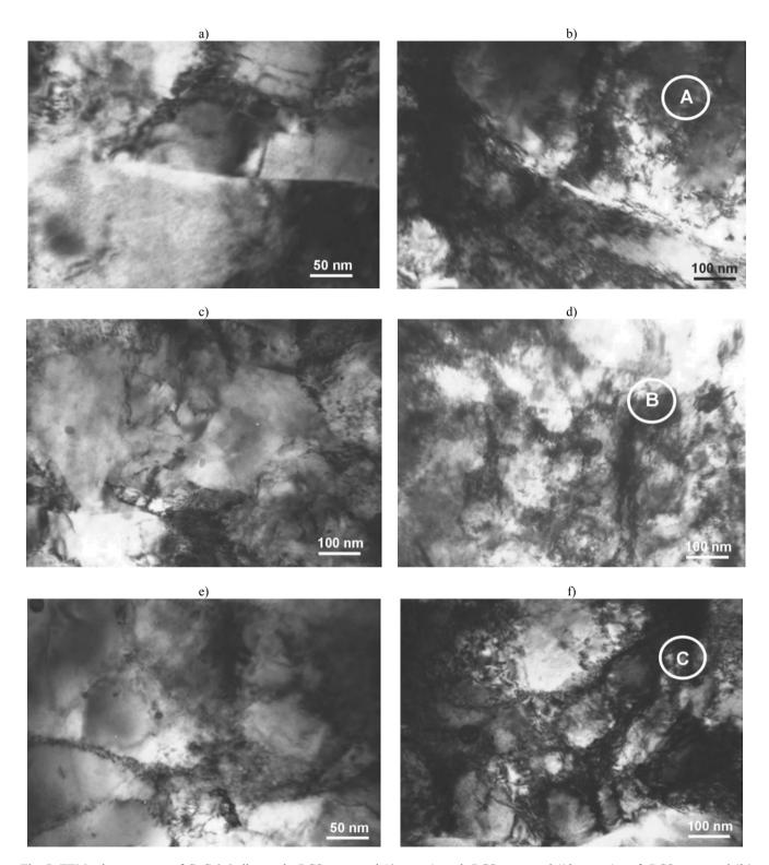
Fig. 7. TEM microstructure of CuCr0,6 alloy; a, b- RCS processed (6 passes), c, d- RCS processed (12 passes), e, f- RCS processed (34 passes). Column A of RCS processed samples represents microstructures of thin foils parallel to the strip surface and column B of RCS processed samples show microstructures of thin foils perpendicular to the strip surface and along the strip
