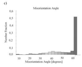
Fig. 4. Microstructure of as-annealed CuCr0,6 alloy strip (EBSD): a- IQ map, b- grain size distribution, c- misorientation angle distribution
