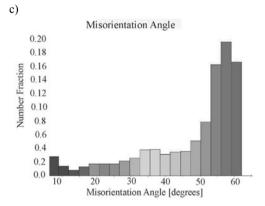
Fig. 5. Microstructure of CRCS processed (34 passes) strips of CuCr0,6 alloy (EBSD); a- IQ, b- grain size distributions, c-misorientation angle distribution
