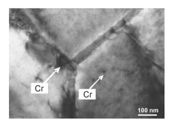
Fig. 6. Microstructure of as annealed (650  $^{\circ}\text{C/1hr}$ ) CuCr0,6 alloy strip –TEM
