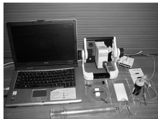
Fig. 4. Measurement equipment for piezoelectric foil tests.
