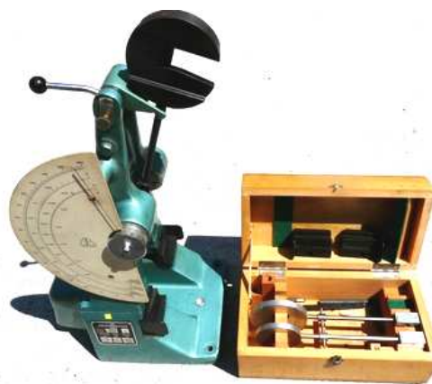
Fig.13. Charpy Hammer long with the instrumentation.
