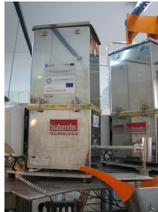
Fig.4. Filling the gravimetric feeders.
