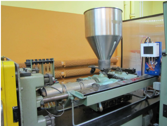
Fig.8. Setting the parameters of injection molding machines used to prepare samples for testing the mechanical parameters of the composite.
