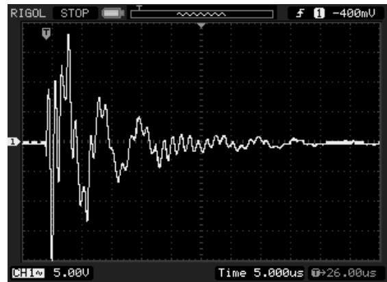
Fig.4. Example waveform on the output high voltage pulses generator
