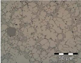
Fig. 9. Microstructure of the AlSi9Cu3 alloy, high pressure cast
