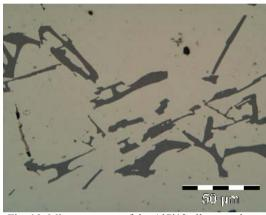
Fig. 10. Microstructure of the AlSi12 alloy, sand cast
