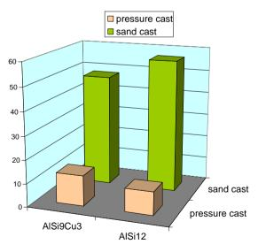
Fig. 6. Results of the anodic layer thickness measurement
