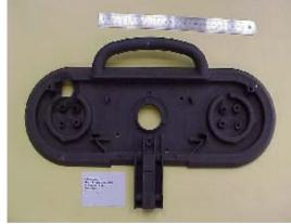
Fig. 5. Overanodized element made from the AC-AlSi9Cu3 aluminium alloy, produced by the Pressure Cast method
