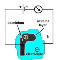
Fig. 1. Scheme of the anodization process including the anodized part, electrolyte, power supply and the alumina surface layer.
