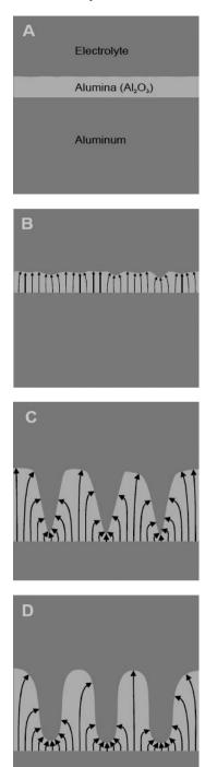
Fig. 2. Stages in the development of the alumina surface layer, a) barrier layer development, b) growth of small inhomogenities, c) continuously grow of pores, d) stabilization of the interpore distances (JPK Instruments AG, 2003).
