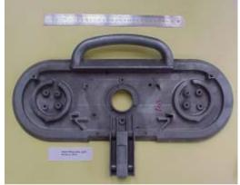
Fig. 4. Anodized element made from the AC-AlSi9Cu3 aluminium alloy, produced by the Pressure Cast method
