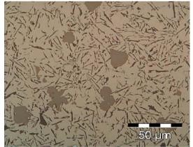
Fig. 11. Microstructure of the AlSi12 alloy, high pressure cast
