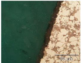
Fig. 7. Anodic alumina layer generated on the AlSi9Cu3 alloy, high pressure cast
