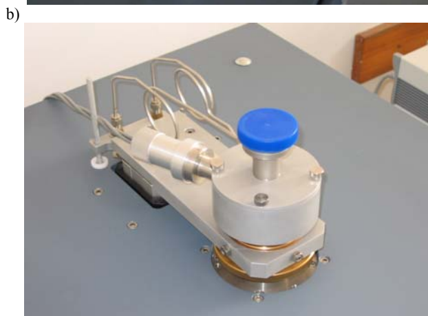
Fig. 1. A multi HTCS calorimeter: a) a view of crucible, b) measuring head [4]
