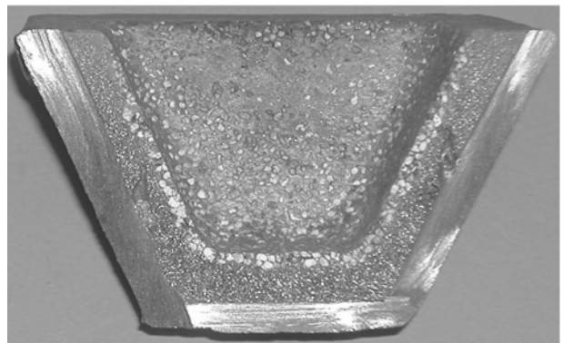
Fig. 4. View of cross-section of cast iron ingot mould with composite surface layer on the basis of SiO_2
