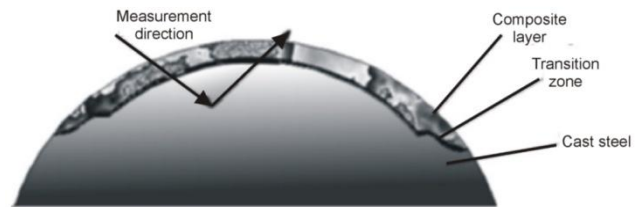
Fig. 2. Scheme of hardness measurement on cross-section of test casting of sphere
