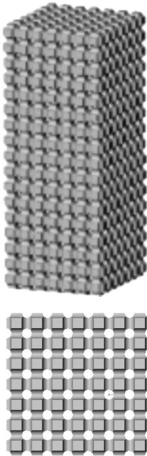
Fig.1. Geometry of the cores for skeleton casting manufacturing (casting negative)
