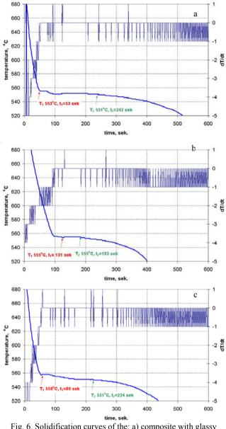
Fig. 6. Solidification curves of the: a) composite with glassy carbon (Cg) particles, b) composite with silicon carbide ceramic particles (SiC), b) AlSi12CuMgNi/SiC<sub>p</sub>+Cg heterophase composite.
