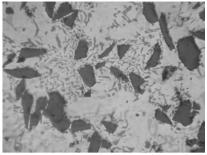
Fig. 4. Microstructure of AlSi12CuMgNi/SiC<sub>p</sub> composite ingot.
