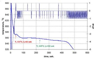
Fig. 5. Solidification curve of the AlSi12CuMgNi aluminium matrix alloy.
