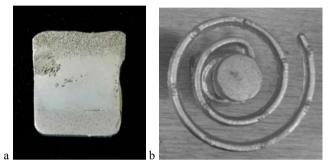
Fig. 2. The AlSi12CuMgNi -SiC<sub>p</sub> + Cg<sub>p</sub> composite material a) macrostructure of composite ingot with particles displacement visible in the matrix, b) spiral test of composite suspension.
