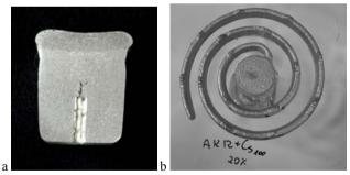
Fig. 1. The AlSi12CuMgNi -Cg<sub>p</sub> composite material: a) macrostructure of composite ingot with particles displacement visible in the matrix, b) spiral test of composite suspension.
