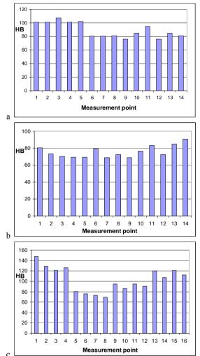
Fig. 7. Brinell' hardness on the cross section of composite ingots:
