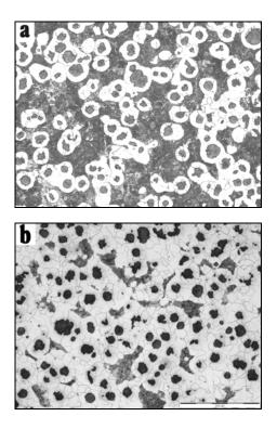
Fig. 5. Microstructure in 5 mm thick casting wall: a) initial state b) after cooling
