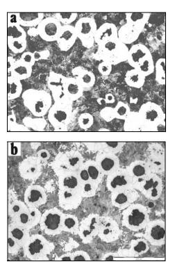
Fig. 7. Microstructure in 15 mm thick casting wall: a) initial state b) after cooling
