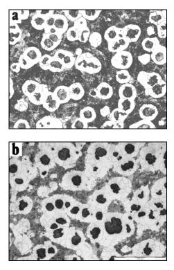
Fig. 6. Microstructure in 10 mm thick casting wall: a) initial state b) after cooling
