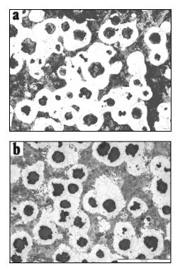
Fig. 8. Microstructure in 20 mm thick casting wall: a) initial state b) after cooling
