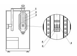
Fig. 2. The schematic diagram of Multi HTC S60 scanning calorimeter
