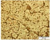
Fig 1. Microstructure alloy with 12 % Al without heat treatment- 0
