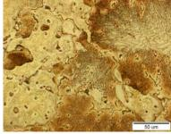
Fig. 4. Microstructure alloy with 12% Al after cooling with the furnace
