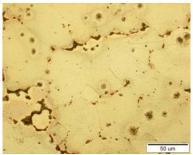
Fig. 2. Microstructure alloy with 12 % Al after cooling in the water
