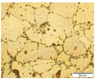
Fig. 3. Microstructure alloy with 12 % Al after cooling in the air
