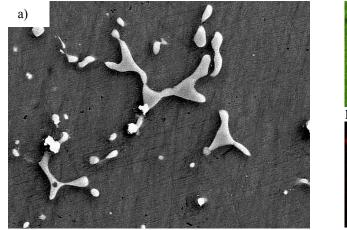
Fig. 10. The area analysis of chemical elements alloy MCMgAl12Zn1 after cooling in the water: image of secondary electrons (a) and maps of elements' distribution
