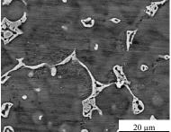
Fig. 6. Microstructure alloy with 12 % Al without heat treatment- 0
