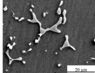
Fig. 7. Microstructure alloy with 12 % Al after cooling in the water
