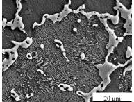
Fig. 8. Microstructure alloy with 12% Al after cooling in the furnace
