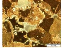
Fig. 5. Microstructure alloy with 12% Al after aging treatment
