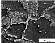
Fig. 9. Microstructure alloy with 12% Al after aging treatment
