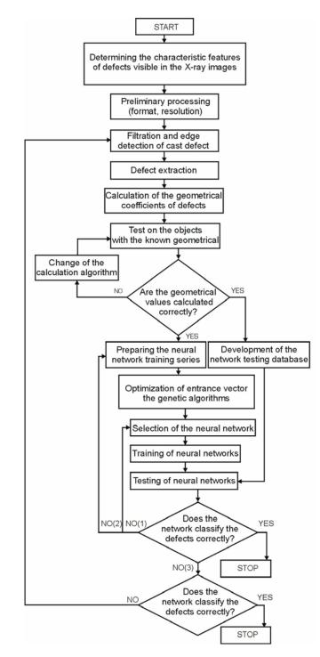
Fig. 2. Block diagram of the developed methodology of data processing pertaining to casting defects observed in the examined castings of the internal combustion engine elements from the Al-Si-Cu alloy
