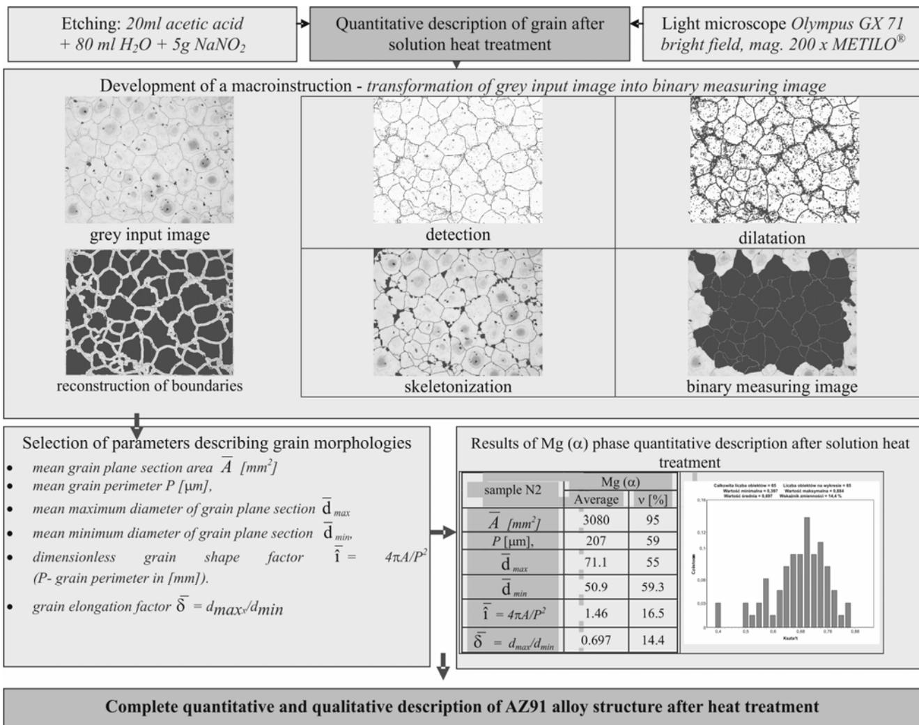
Fig. 5. Chart of the AZ91 alloy structure evaluation procedure, part IV: Quantitative description of Mg(α) phase grain after solution heat treatment
