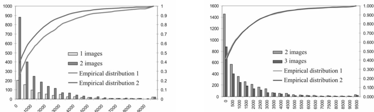
Fig. 6. Distributions of frequency as a function of the grain plane section area, determined for one and two and three measurement fields, and the corresponding empirical distribution functions for the investigated specimen
