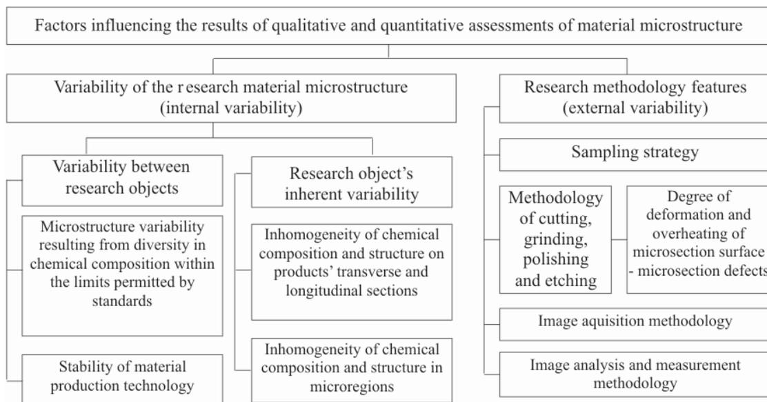
Fig. 1. Factors influencing the results of a qualitative and quantitative evaluation of material structures [8]
