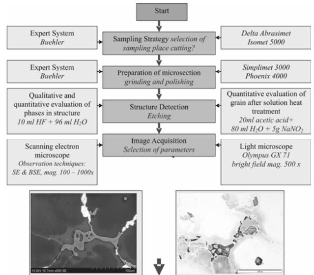
Fig. 2. Chart of the AZ91 alloy structure evaluation procedure, part I: Structure detection [14, 15]
