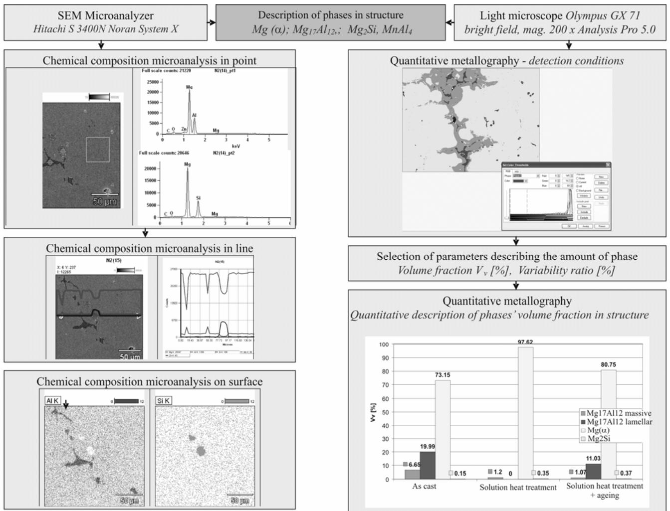
Fig. 4 Chart of the AZ91 alloy structure evaluation procedure, part III: Qualitative and quantitative description of phases
