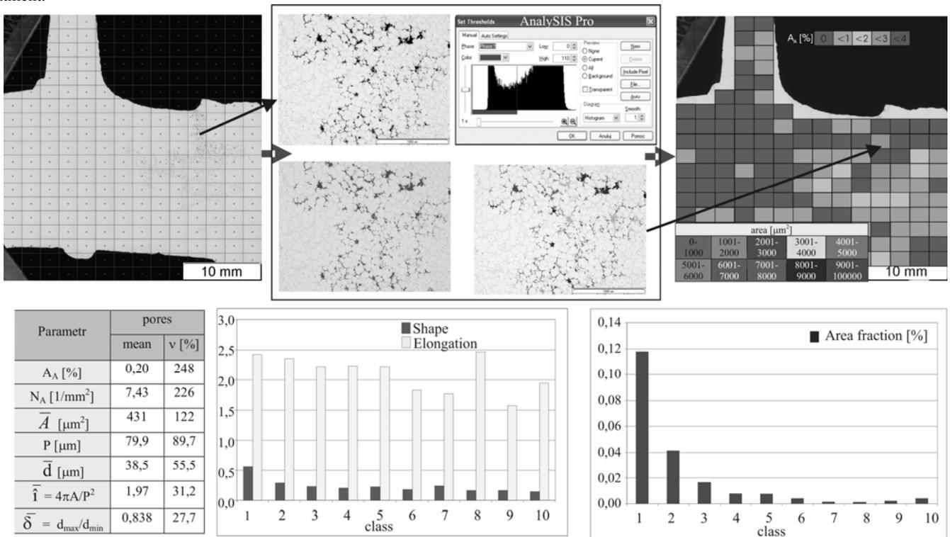
Fig. 3. Chart of the AZ91 alloy structure evaluation procedure, part II: Quantitative description of porosity
