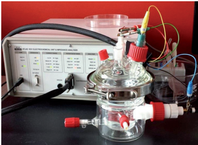
Fig. 2. Electrochemical test stand which consists of a potentiostat and an electrochemical cell
