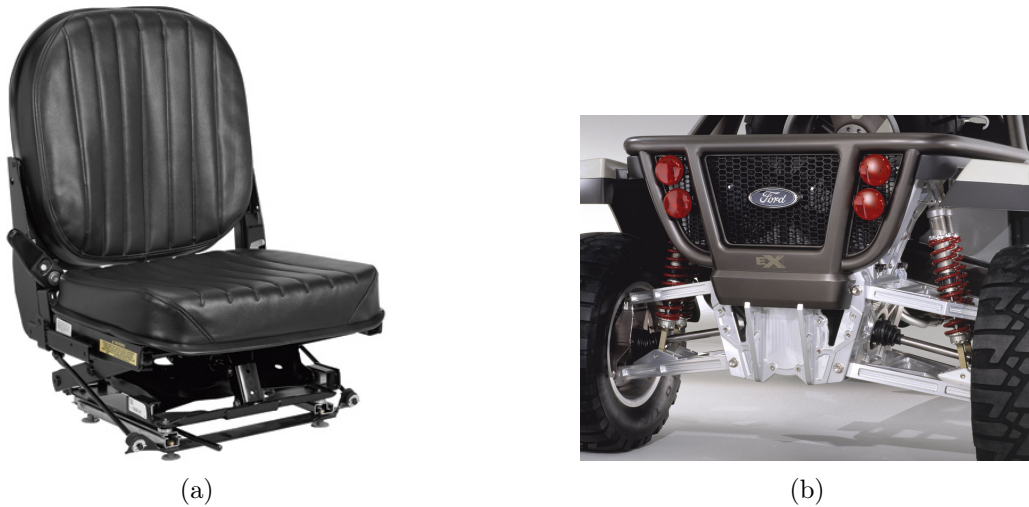
Figure 1.3: Examples of suspension systems in vehicles: a) suspension of passenger seat [155], b) vehicle suspension system [156]
