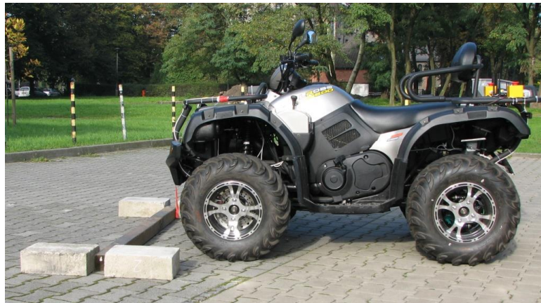
Figure 7.3: Single-road-bump excitation of the experimental vehicle
