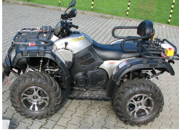
Figure 1.9: An off-road vehicle equipped with suspension MR dampers and semiactive suspension control system
