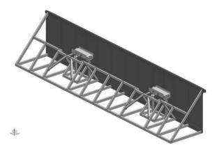
Fig. 6. The strength test of the side walls of the wagon
