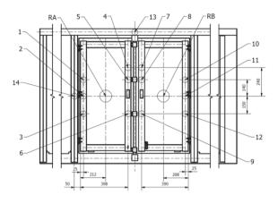
Fig. 15. The distribution and numbering of strain gauges
