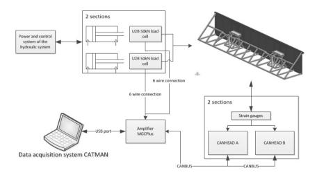
Fig. 9. The measuring circuit
