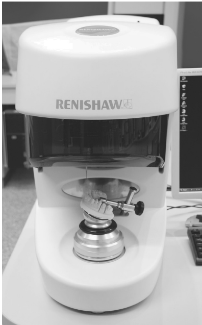
Fig. 4. Dental contacting scanner 3i Incise Renishaw
