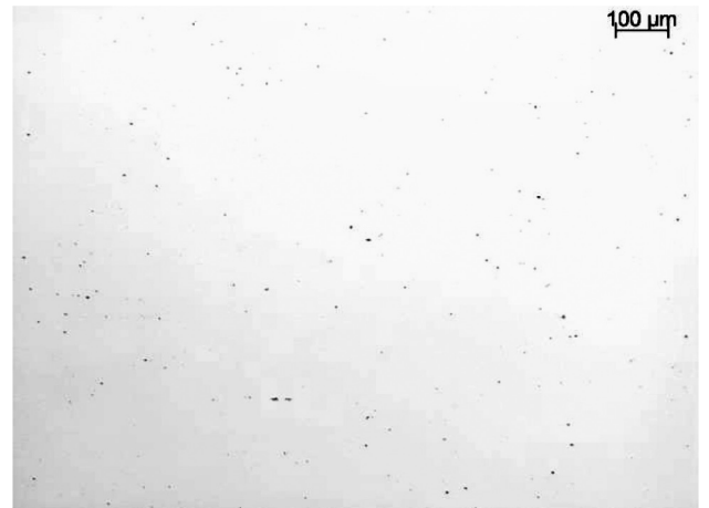
Fig. 3. Distribution of non-metallic inclusions at the longitudinal section of the thermomechanically rolled 5MnNb steel sheet; the steel is modified by mischmetal
