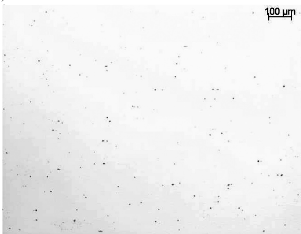
Fig. 2. Distribution of non-metallic inclusions at the longitudinal sections of the thermomechanically rolled sheets; 3Mn steel is not modified by mischmetal (a) whereas 3MnNb steel is modified by mischmetal (b)
