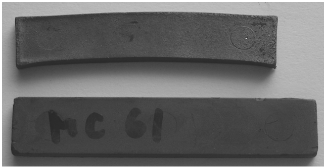
Fig. 8. View of samples after moulding and sintering at the temperature of 1260°C
