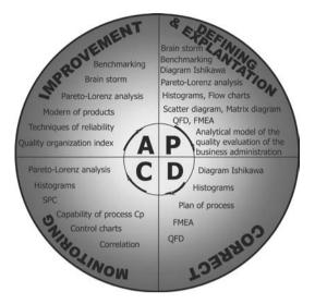
Fig. 1. Model PDCA connects with quality methods and quality tools [7]
