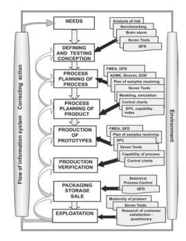
Fig. 5. Model of quality research and estimation methods based on product life cycle [8]
