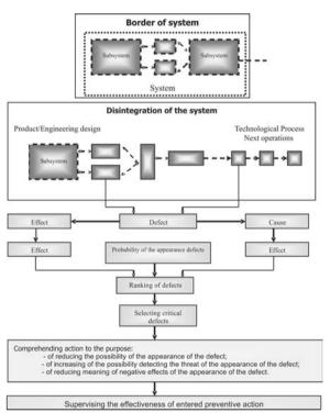
Fig. 6. Stages of FMEA method [20]
