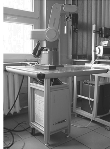
Fig. 12. The RV-M1 robot's manipulator mounted on the stand in the Institute's robotics laboratory. Under the table the controller is mounted
