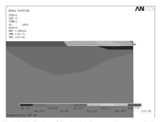
Fig. 14. Distribution of the simulated compression stresses in the single-layer Ti(C,N) coating deposited on to  $Al_2O_3+TiC$  type oxide tool ceramics substrate
