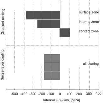
Fig. 18. Schematic distribution of stresses in the (Ti,Al)N coatings deposited on  $Al_2O_3$ +TiC type oxide tool ceramics substrate obtained by computer simulation
