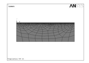
Fig. 1. True model subjected to discretization with deposited gradient and single-layer (Ti,Al)N and Ti(C,N) on different substrates
