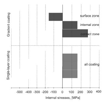
Fig. 19. Schematic distribution of stresses in the Ti(C,N) coatings deposited on cemented carbides obtained by computer simulation
