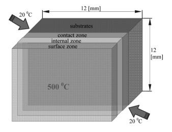
Fig. 2. Real model of gradient coatings
