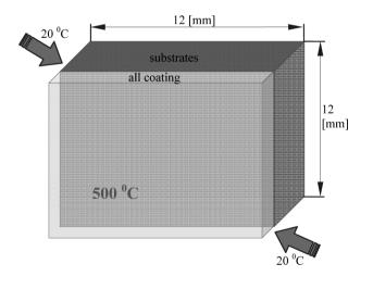
Fig. 3. Real model of single-layer coatings
