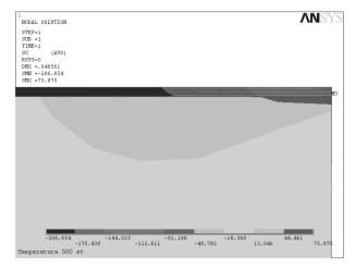
Fig. 8. Distribution of the simulated compression stresses in the single-layer (Ti,Al)N coating deposited on to  $Al_2O_3$ +TiC type oxide tool ceramics substrate
