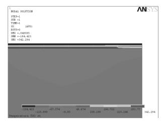
Fig. 15. Distribution of the simulated compression stresses in the gradient Ti(C,N) coating deposited on to  $Al_2O_3$ +TiC type oxide tool ceramics substrate
