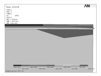
Fig. 7. Distribution of the simulated compression stresses in the gradient (Ti,Al)N coating deposited on to cermet substrate
