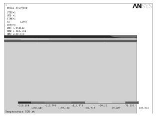
Fig. 13. Distribution of the simulated compression stresses in the gradient Ti(C,N) coating deposited on to cermet substrate
