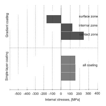
Fig. 21. Schematic distribution of stresses in the Ti(C,N) coatings deposited on  $Al_2O_3$ +TiC type oxide tool ceramics substrate obtained by computer simulation
