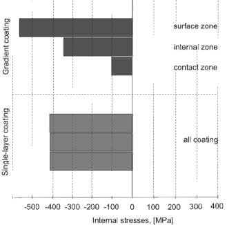
Fig. 17. Schematic distribution of stresses in the (Ti,Al)N coatings deposited on cermet substrates obtained by computer simulation
