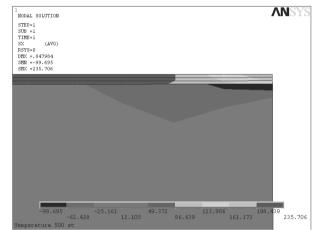
Fig. 10. Distribution of the simulated compression stresses in the single-layer Ti(C,N) coating deposited on to cemented carbide substrate
