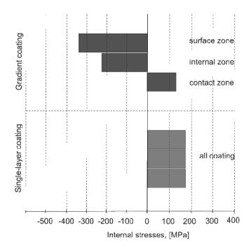
Fig. 16. Schematic distribution of stresses in the (Ti,Al)N coatings deposited on cemented carbides obtained by computer simulation
