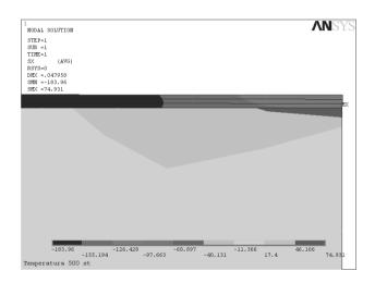
Fig. 4. Distribution of the simulated compression stresses in the singlelayer (Ti,Al)N coating deposited on to cemented carbide substrate
