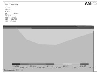
Fig. 9. Distribution of the simulated compression stresses in the gradient (Ti,Al)N coating deposited on to  $Al_2O_3$ +TiC type oxide tool ceramics substrate
