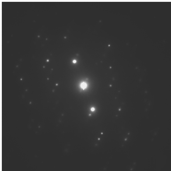
Fig. 12. Structure of cermet substrate: a) bright field; b) dark field from (\bar{2}00) TiC i (11\bar{1}) Co reflex; c) diffraction pattern from area b and d) solution of the diffraction pattern
