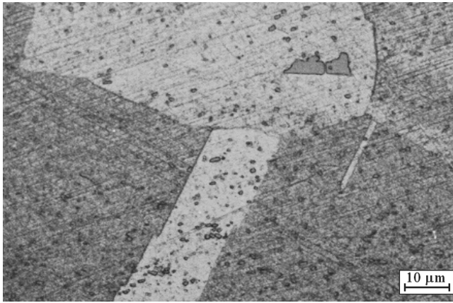
Fig. 10. Large grains in the matrix-α with precipitations in the alloy CCNB after solution heat treatment from 1000°C
