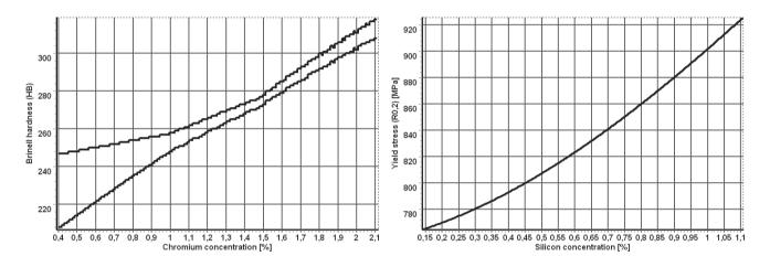
Fig. 7. Influence of chromium concentration on Brinell hardness and silicon concentration on yield stress based on 41Cr4 steel
