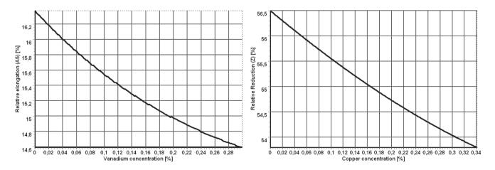
Fig. 5. Influence of vanadium concentration on relative elongation and copper concentration on relative area reduction based on 34CrNiMo6 steel
