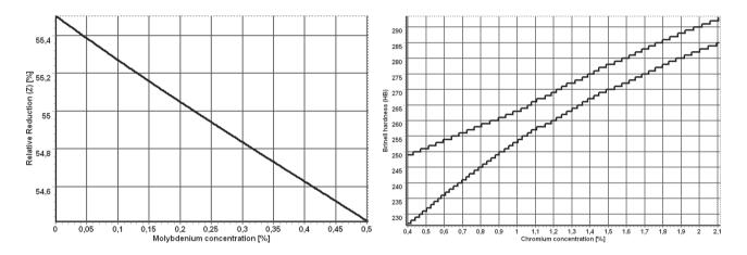
Fig. 10. Influence of molybdenium concentration on relative area reduction and chromium concentration on Brinell hardness based on 42CrMo4 steel
