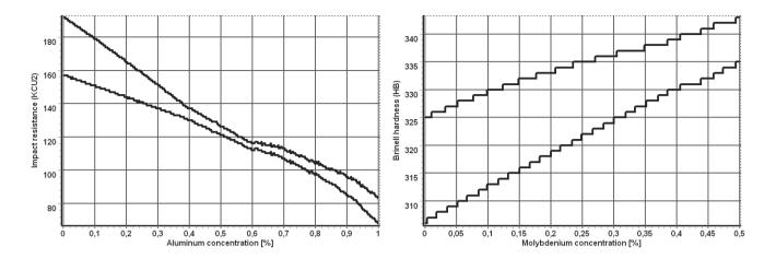
Fig. 6. Influence of aluminium concentration on impact resistance and molybdenum concentration on Brinell hardness based on 34CrNiMo6 steel
