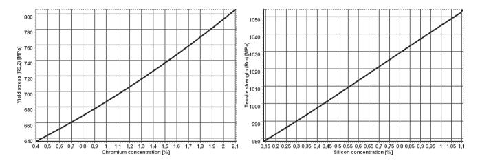
Fig. 3. Influence of chromium concentration on yield stress and silicon concentration on tensile strength based on 30CrMo5-2 steel
