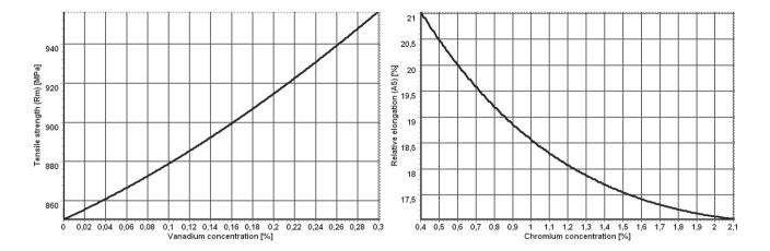
Fig. 9. Influence of vanadium concentration on tensile strength and chromium concentration on relative elongation based on 42CrMo4 steel
