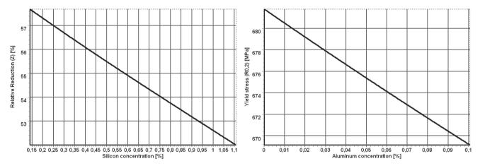
Fig. 1. Influence of silicon concentration on relative area reduction and aluminium concentration on yield stress based on 24CrMo4 steel
