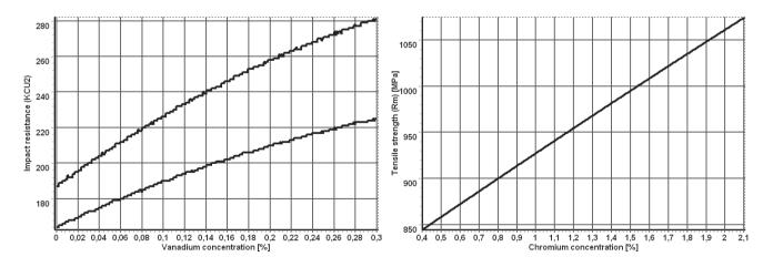
Fig. 8. Influence of vanadium concentration on impact resistance and chromium concentration on tensile strength based on 41Cr4 steel
