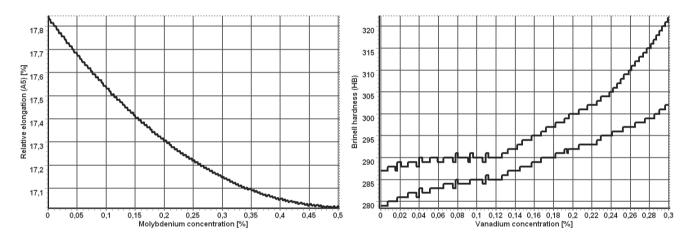
Fig. 4. Influence of molybdenum concentration relative elongation and vanadium concentration on Brinell hardness based on 30CrMo5-2 steel
