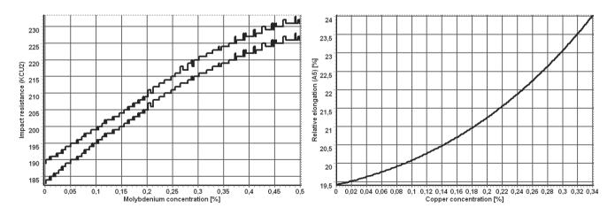
Fig. 2. Influence of molybdenium concentration on impact resistance and copper concentration on relative elongation based on 24CrMo4 steel
