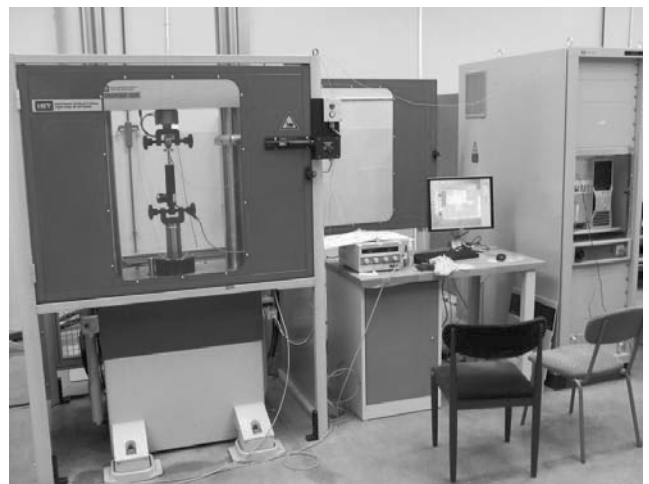
Fig. 1. A servo-hydraulic test-rig used in experimental investigations
